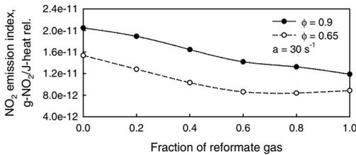
Fig. 7. Variation of  $\text{NO}_2$  emission index.
