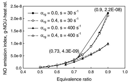
Fig. 6. Variation of NO emission index with equivalence ratio.
