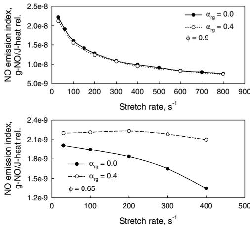
Fig. 5. Effect of stretch rate on NO formation.
