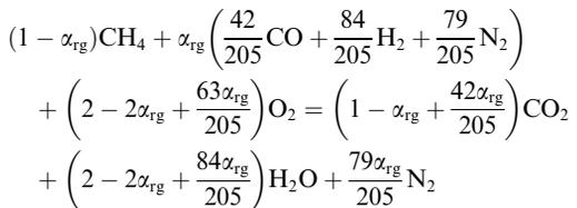
Nitrogen in this reaction is from the fuel reforming, while that contained in air does not explicitly appear here, since it does not affect the calculation of fuel–oxidant ratio. Therefore, the stoichiometric fuel–oxidant ratio in a reformat gas enriched mixture is:
