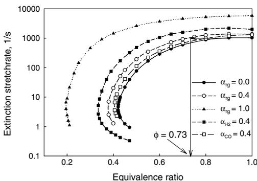
Fig. 1. Effect of the addition of reformat gas, H<sub>2</sub> and CO on C-shaped curves.
