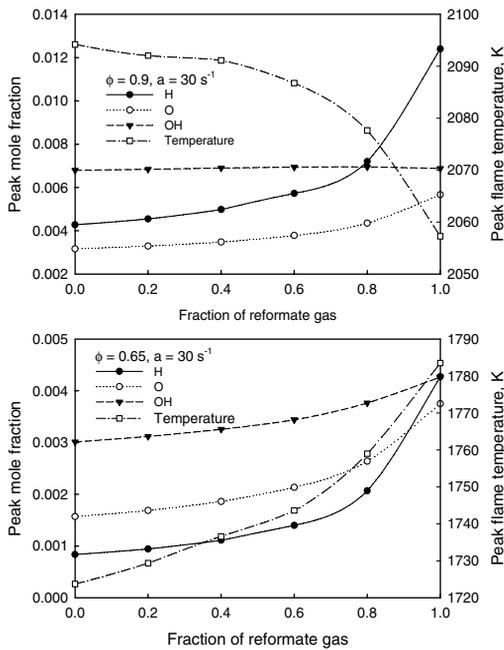
Fig. 4. Variations of peak temperature and peak mole fractions of H, O, and OH.
