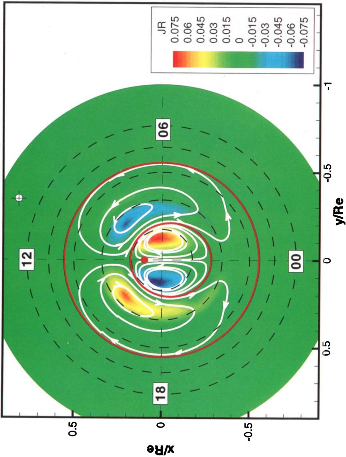
**Plate 2.** Simulation results for the northern polar ionosphere for the reference run shown in Plate 1. The color code represents the radial component of the current density with red denoting upward and blue representing downward currents. The white lines with arrowheads are convection streamlines. The thick red circles separate regions of distinct flow characteristics. The red dot indicates the ionospheric footprint of the reconnection point shown in Plate 1a.
