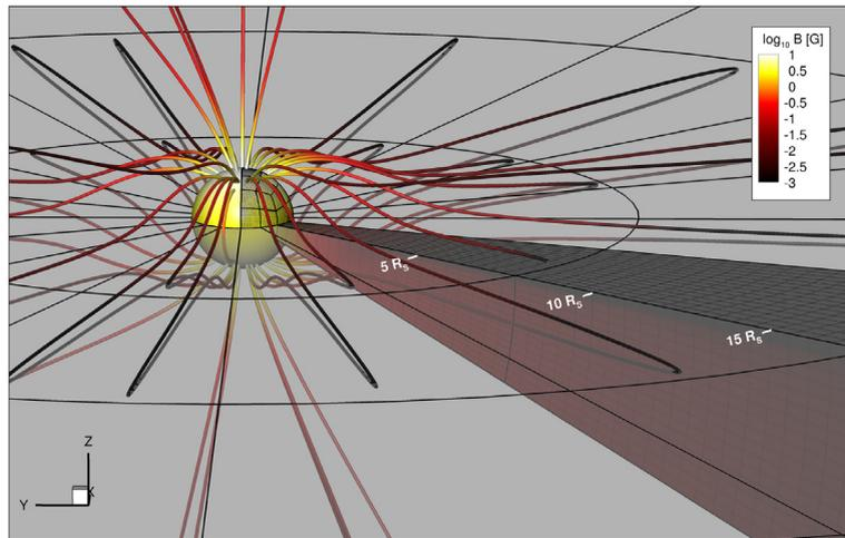
**Fig. 15.** Three-dimensional representation of open and closed magnetic field lines in the corona region. Two blocks of the cubed-sphere grid and the associated meshes are completely shown together with the edges of the blocks in the equatorial plane and the edges and face nodes of several blocks at the inner sphere.
