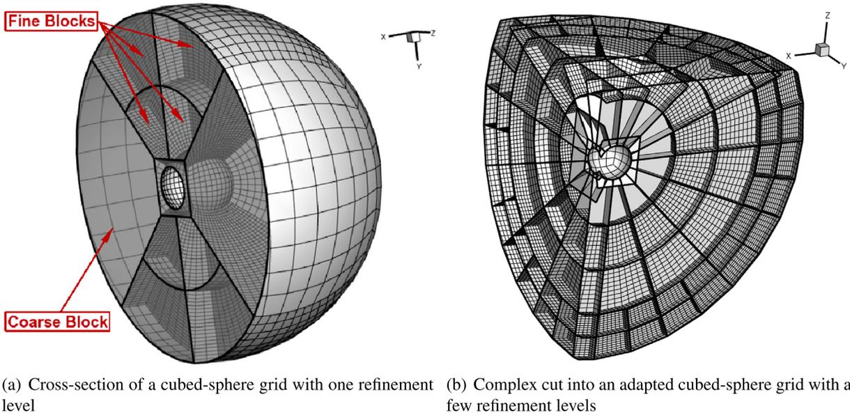
Fig. 5. Illustration of three-dimensional block-based adapted cubed-sphere grids showing the block boundaries and the associated meshes.
