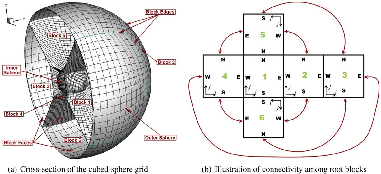
**Fig. 1.** Three-dimensional cubed-sphere grid with six root blocks (corresponding to the six sectors of the grid) and depiction of inter-block connectivity. In our approach, the root blocks can be refined in a block-adaptive way. In panel (b), the block faces are denoted with the initials of the cardinal directions: North (N), East (E), South (S) and West (W).
