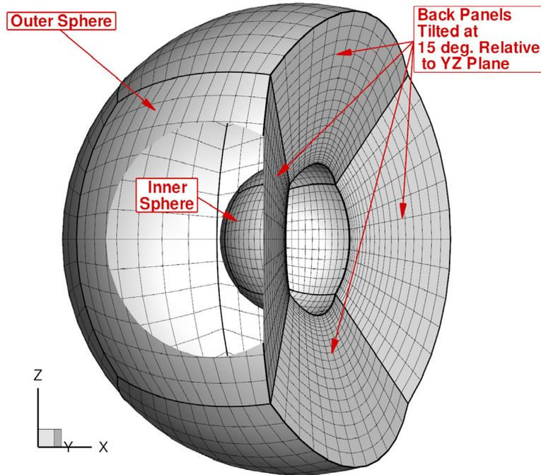
Fig. 12. Cubed-sphere grid formed by only five root blocks, for simulation on one side of the sphere. A cut in the outer spherical geometry allows a better view of the inner spherical cap.
