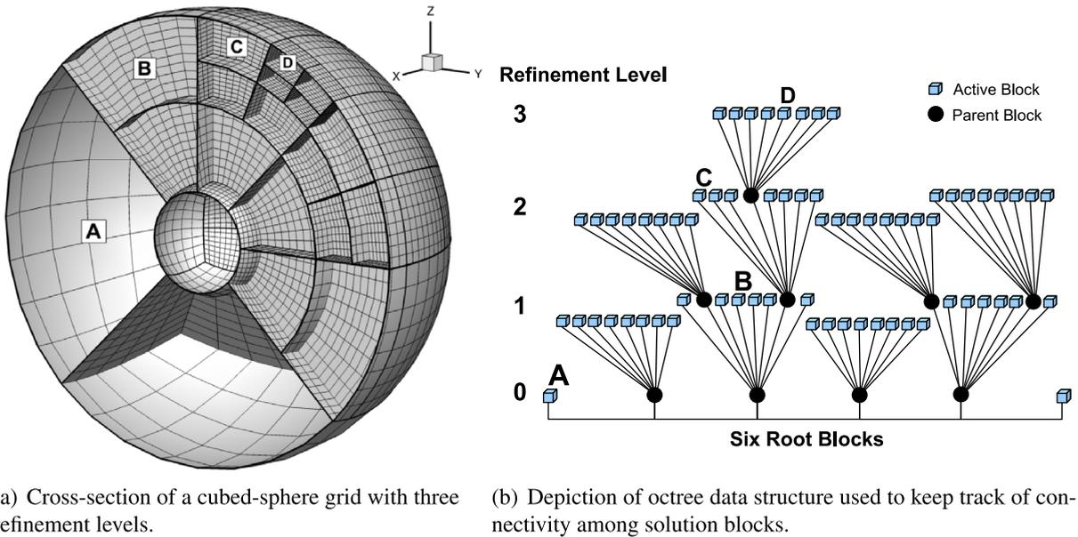
Fig. 3. Illustration of three-dimensional block-based adapted cubed-sphere grids showing the blocks and block boundaries.
