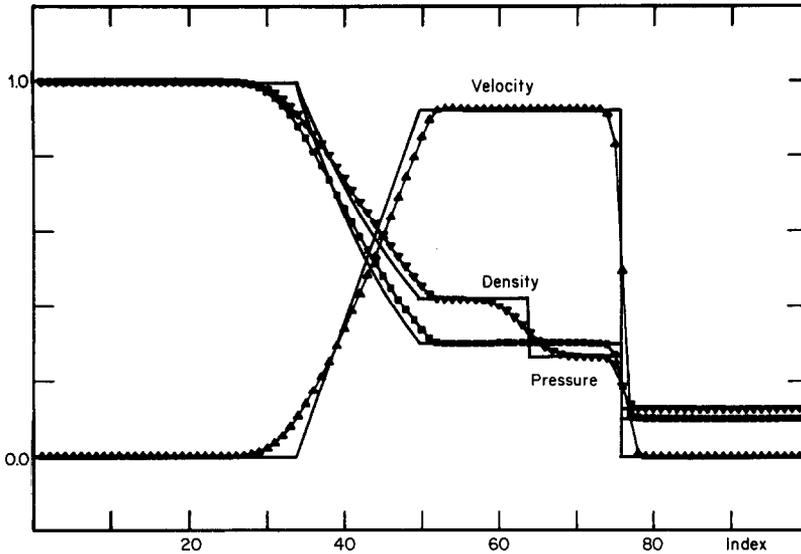
FIG. 2. Numerical solution to a shock-tube problem, incorporating either the exact or the approximate Riemann solution in a first-order upwind difference scheme.
