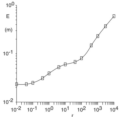
Fig. 10 Periodicity error measure (10 orbits) versus LQR control weighting  $r$
