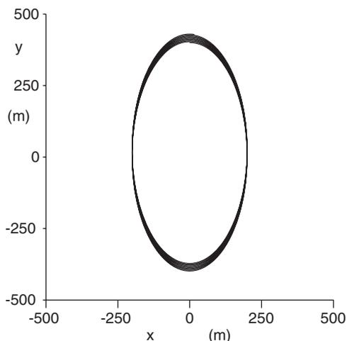
Fig. 12  $J_2$ -invariant ICs with errors (10 orbits)
