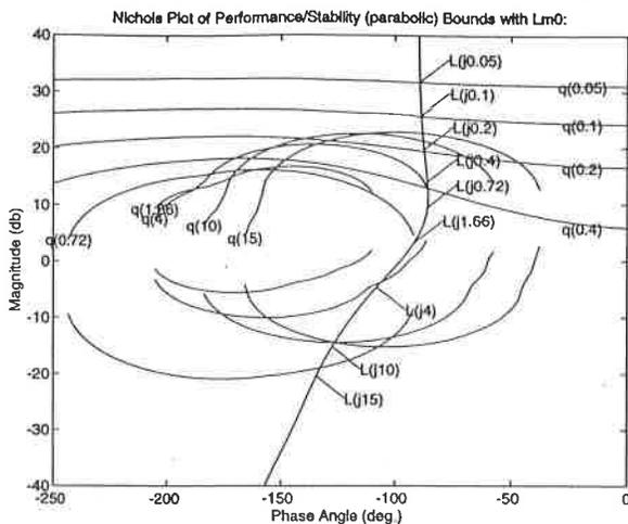
Fig. 1 Nichols Chart plot (log magnitude-phase) of open loop tracking bounds  $q(\omega)$  for the Example of Eq. (17) including the minimum phase nominal loop transmission function  $L_{m0}(j\omega)$  (labeled  $L(\omega)$  in the figure) based upon the initial feasible controller of Eq. (19)
