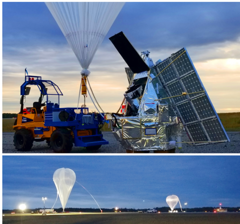
FIG. 3. SUPERBIT pre-launch 2019 (site: Timmins, Ontario); during inflation of the primary balloon (bottom left), SUPERBIT is secured by the launch support vehicle (top) beneath the smaller tow balloon (bottom right); on launch, the tow balloon provides neutral buoyancy for the payload as the primary balloon is released and ascends above it.
