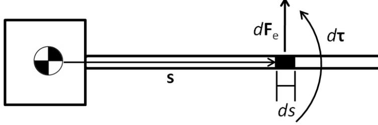
The electrodynamic torque  $\boldsymbol{\tau}_{jm}$  acting on the  $j^{\text{th}}$  boom can be calculated by integrating  $d\boldsymbol{\tau}_{jm}$  over the length of the boom such that,
