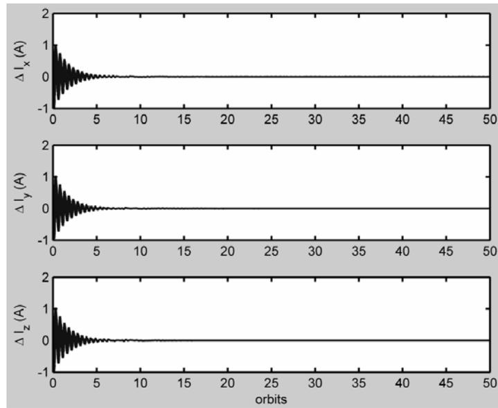
For the last example, consider an equatorial satellite with the control gains set as  $K_d = 5,000$  A · s/Wb and  $K_p = 0.1$  A/Wb. Figure 10 shows that the electrodynamic booms are unable to align the satellite’s body axes with the ECI frame even after 300 orbits. This is because the available torque about the  $\mathbf{x}_B$  and  $\mathbf{y}_B$  axes decreases as the spacecraft
