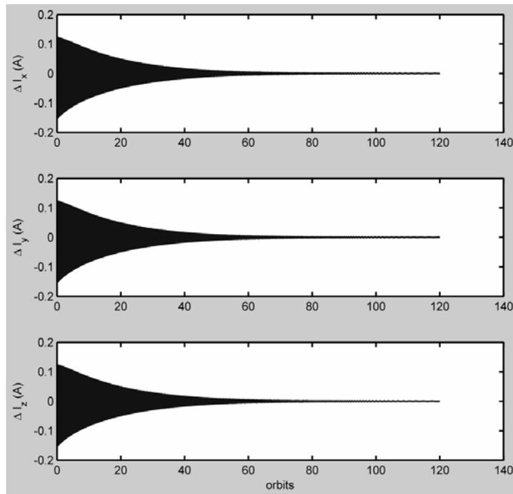
**Figure 6** Satellite detumbling,  $i = 0$  deg,  $K_d = 4,000$  A · s/Wb
