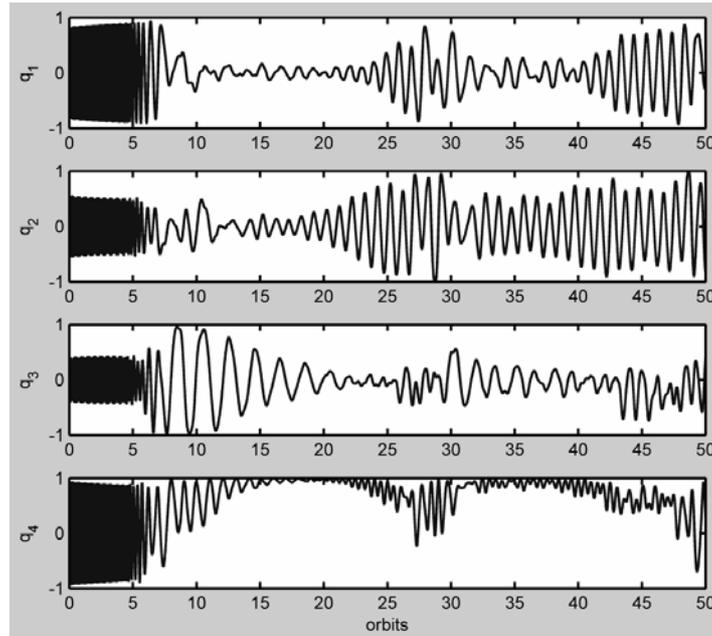
**Figure 10** Satellite in equatorial orbit,  $K_d = 5,000$  A · s/Wb,  $K_p = 0.1$  A/Wb
