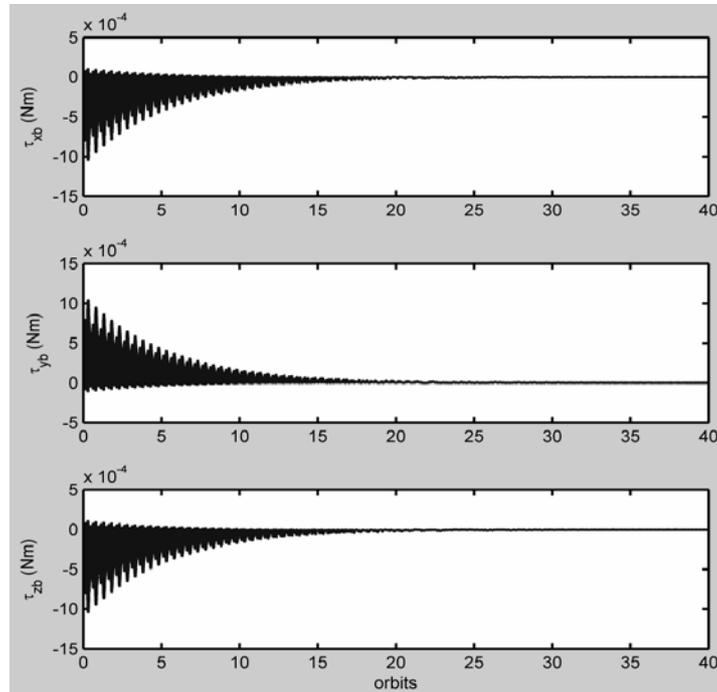
**Figure 5** Satellite detumbling,  $i = 0$  deg,  $K_d = 1,500$  A · s/Wb
