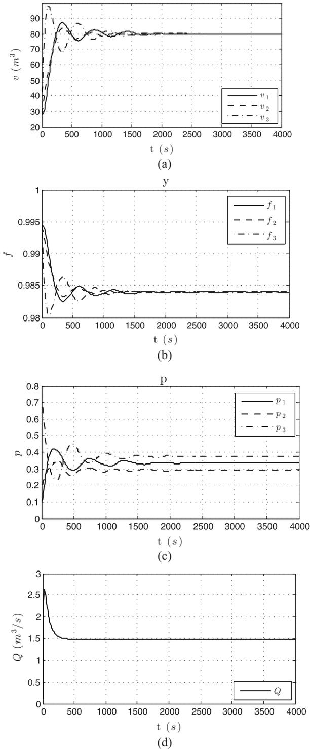
**Figure 9.** Tank system with BNN dynamic (initial condition 1). (a) Tank volumes vs. time; (b) payoffs vs. time; (c) population state vs. time; (d) total input flow vs. time
