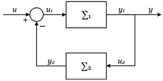
Figure 1. Negative feedback interconnection of two systems.
