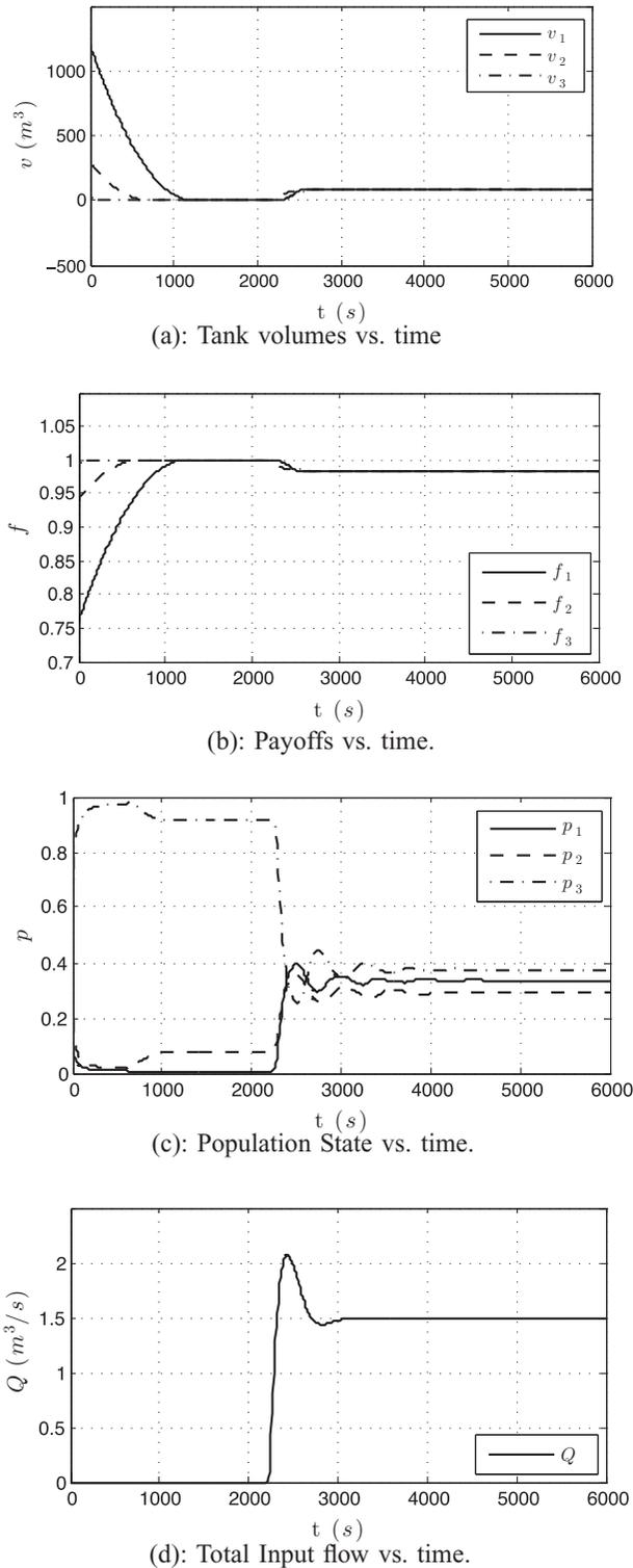
**Figure 11.** Tank system with BNN dynamic (initial condition 2).
