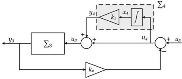
**Figure 7.** Integrator and the gradient controller,  $\Sigma'_3$ .
