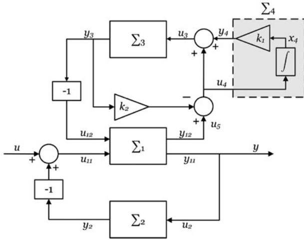
**Figure 6.** Interconnected system with added integrator.
