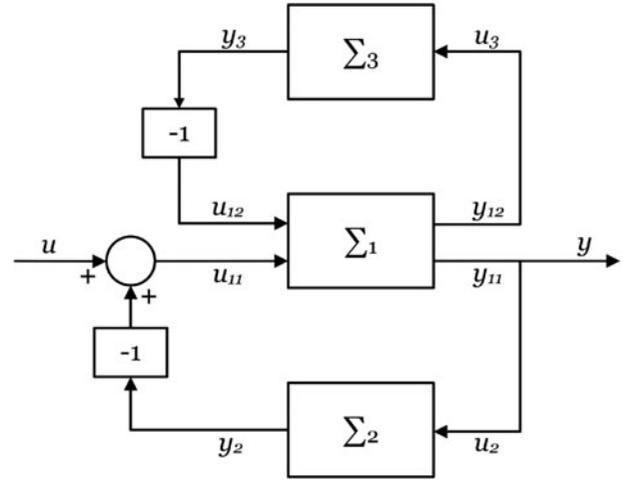
Figure 5. Interconnected system with gradient controller.
