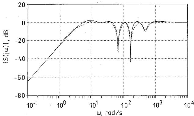
**Fig. 6** Controller properties: sensitivity against frequency
