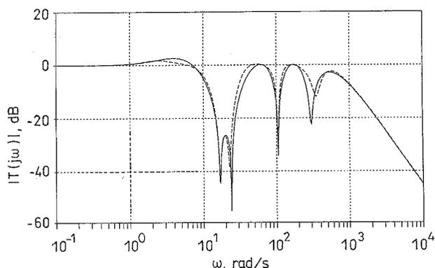
**Fig. 7** Controller properties: complementary sensitivity against frequency
