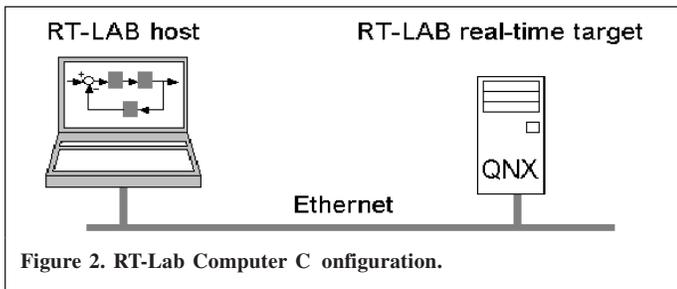
The first computer is the host computer of the RT-Lab system. It has Windows NT as its operating system and runs the RT-Lab software. It is from this machine that the user creates the model that will be simulated in real-time. The host machine is also used to display and store data collected during the simulation run. The user can also interact with the model on the host machine by giving it input either before the simulation is started or while the simulation is running.
