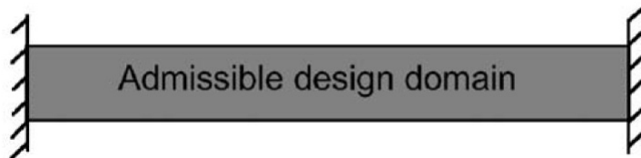
Figure 3.3: Beam constrained at both ends. Figure is adopted from Du and Olhoff [18].
