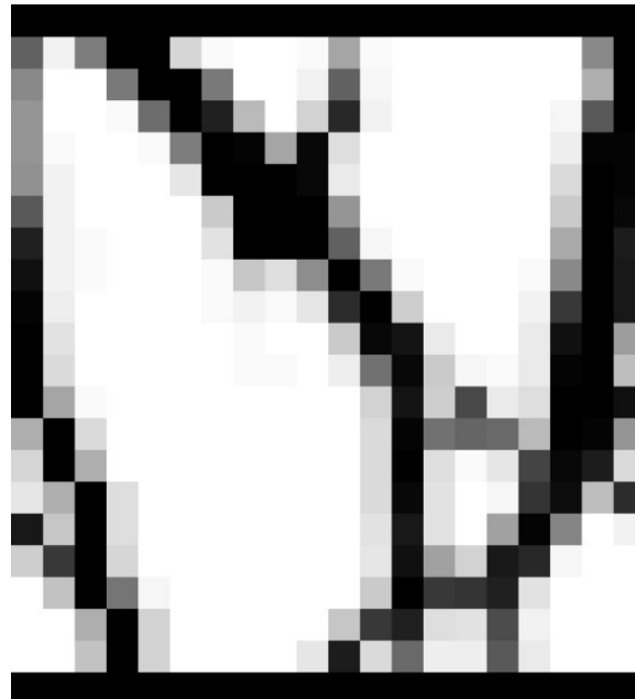
(a) Unit cell of the optimized design with a 22x20 grid size.
