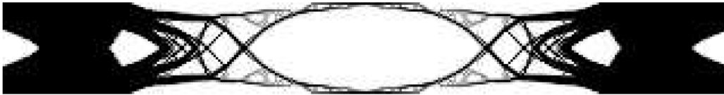
Figure 4.4: Optimized structure with the minimum eigenvalue maximized. \omega_{1max} = 457.6 rad/s with a 40 x 320 grid size, without post-processing.
