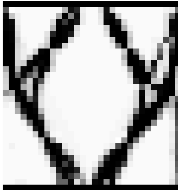
(a) Unit cell of the optimized design with a 32x30 grid size.
