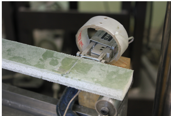
Figure 4.6: Test setup for clip gauge
