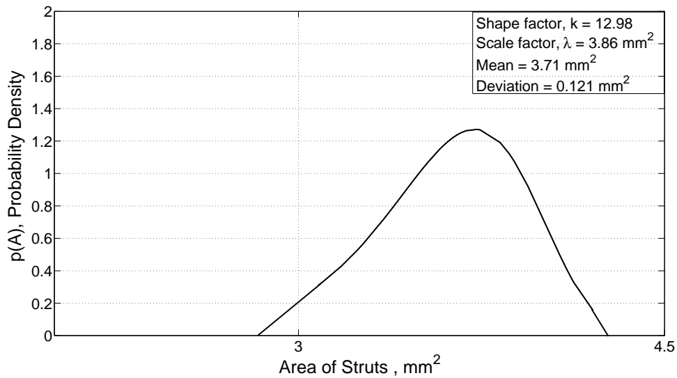
Figure 3.7: Weibull probability density against the cross-sectional area distribution in the 42 struts of the Shear Specimen.
