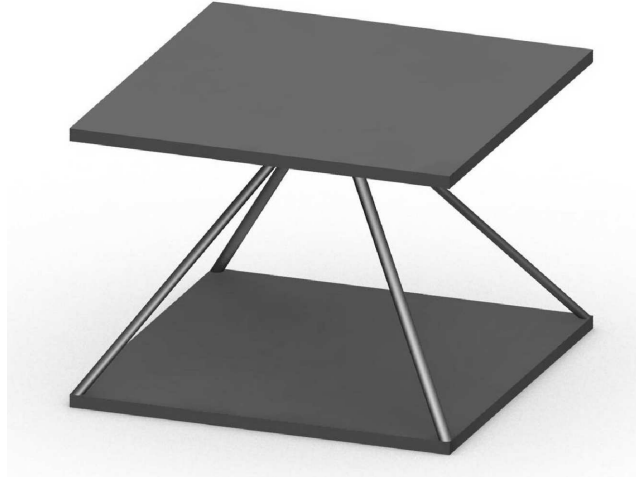
Figure 2.1: Unit cell pyramidal truss sandwich made of circular cylindrical struts. Figure courtesy of John Hwang.
