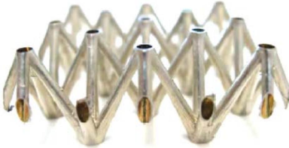
Figure 8.8: Example of a fabrication route to making hollow metallic microtrusses for cores in sandwich panels, taken from Ref. [152].
