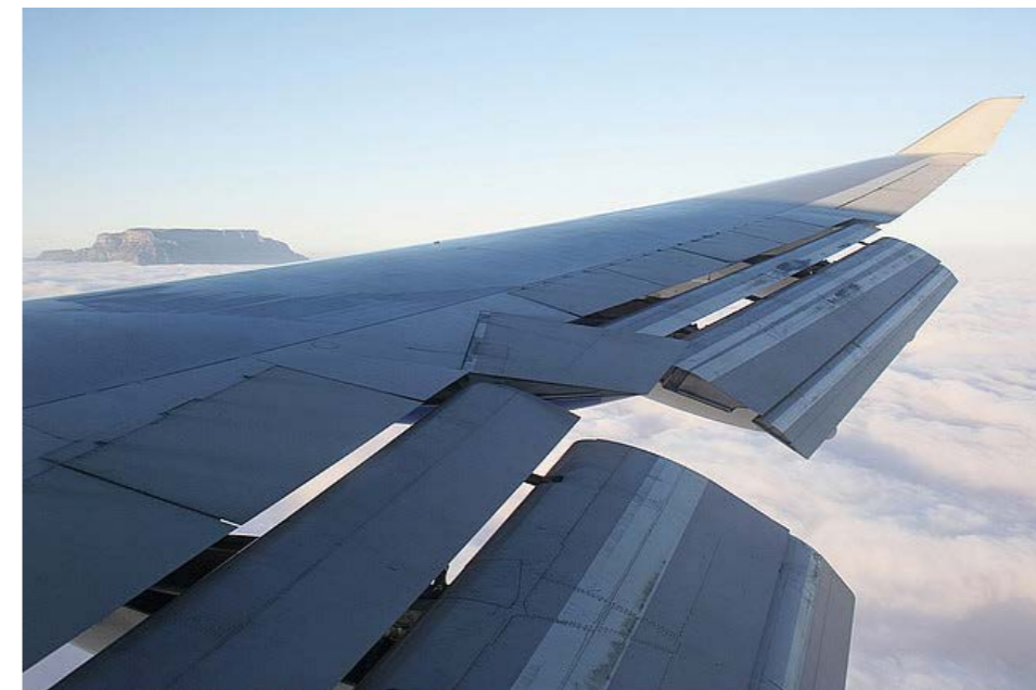
Slotted Fowler flaps of a Boeing 747.
