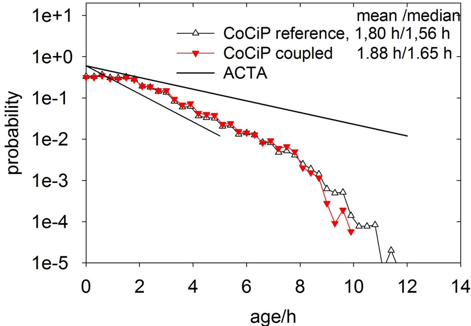
ACTA: upper and lower bounds of contrails tracked with the ACTA algorithm in infrared Meteosat data (Vazquez-Navarro et al., 2015)
