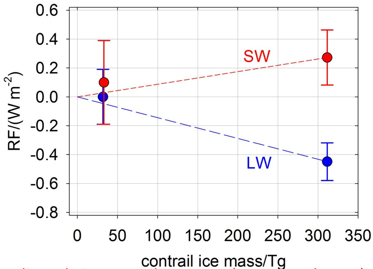
Interpolating linearly in contrail ice mass (Water exchange) suggests a RF from dehydration of order  $\pm 0.04$  (net -0.01)  $W m^{-2}$  for normal traffic
