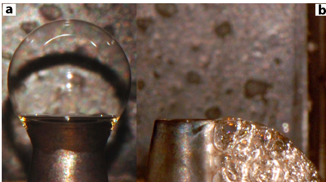
Figure 3. Liquid bubbles at 6.1 and 9.1 MPa. (a) P = 6.1 MPa. Clear and transparent liquid bubble with a diameter of approximately 6.5 mm. (b) P = 9.1 MPa. Small broken liquid bubbles spilled to the side of the fuel nozzle.
