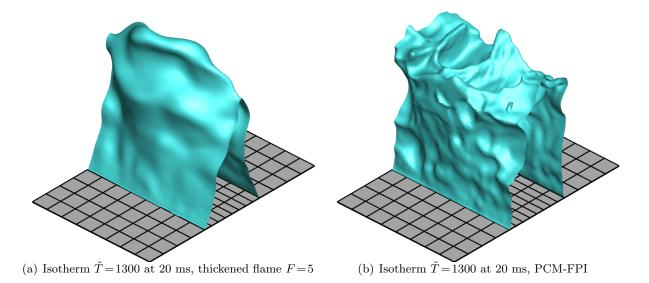
Figure 6.14: Instantaneous flame isotherms for the LES simulations of the Bunsen flame on a slot burner at 20 ms.
