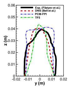
Figure 6.16: Flame brush contour  $\langle c_{\rm T} \rangle = 0.5$  for the present LES and the DNS and experiment reported in Reference [261].
