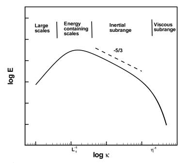
Figure 2.3: Schematic of the turbulent kinetic energy spectrum.
