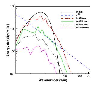
**Figure 6.7:** Evolution of the turbulence kinetic energy spectrum for the decay of homogeneous isotropic turbulence case.
