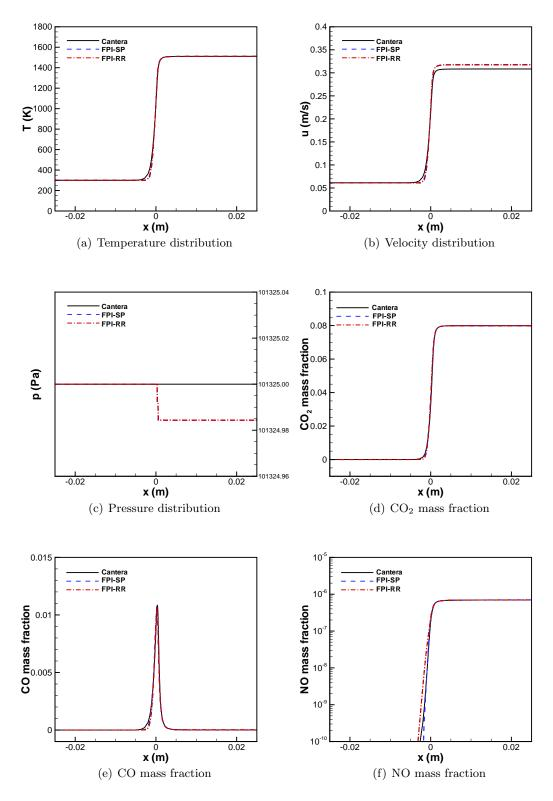
Figure 6.24: Temperature, velocity, pressure, and CO<sub>2</sub>, CO, and NO mass fraction profiles of a 1D steady-state CH<sub>4</sub>-air flame at  $\phi = 0.52$ , corresponding to the PCM-FPI model with  $Y_c = Y_{CO_2} + Y_{NO}$  and 13 species. FPI-SP: reading mass fractions directly. FPI-RR: transporting the species using reconstructed reaction rates.
