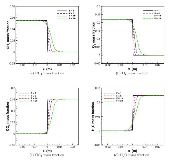
Figure 6.3: Structure of 1D steady-state stoichiometric methane-air thickened flames.
