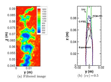
Figure 6.21: Instantaneous filtered temperature from the experiment and 0.5 contour of the averaged  $c_{\rm T}$  map from the experiment and the simulations. Bunsen burner configuration.
