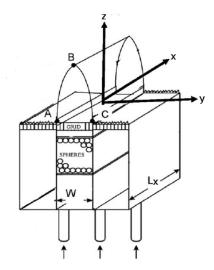
Figure 6.13: Schematic of slot burner showing flame configuration and piloted coflows [260].
