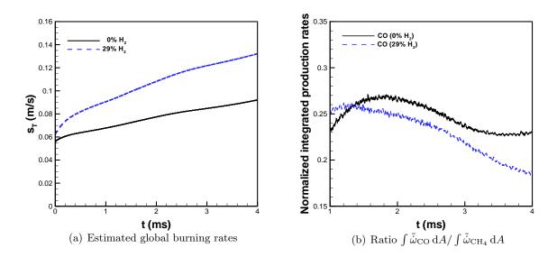
Figure 6.29: Estimated global turbulent flame speeds based on the integrated  $\tilde{\omega}_{Y_c}$  term and integrated CO production rate per integrated CH<sub>4</sub> consumption rate for 2D freely-propagating CH<sub>4</sub>-air and H<sub>2</sub>-CH<sub>4</sub>-air flames. The H<sub>2</sub>-CH<sub>4</sub>-air mixture contained 29% H<sub>2</sub> in the blended fuel.
