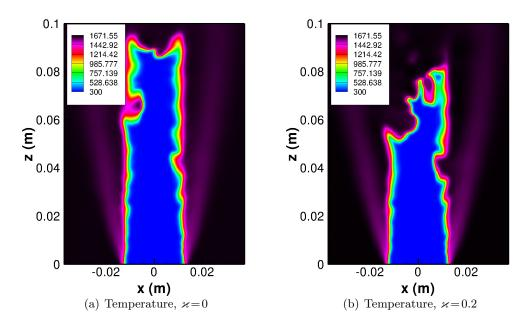
Figure 6.32: Temperature planar cuts of the Bunsen-type flames at 56 ms. Plane y=0. Left: CH<sub>4</sub>-air flame. Right: H<sub>2</sub>-CH<sub>4</sub>-air flame.
