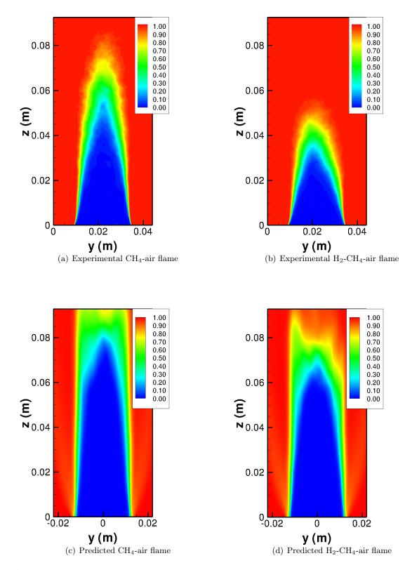
Figure 6.35: Comparison of experimental and predicted temperature-based flame brushes for the Bunsen-type  $CH_4$ -air and  $H_2$ - $CH_4$ -air flames.
