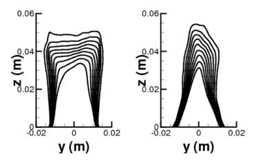
Figure 6.18: Flame brushes corresponding to the thickened flame and PCM-FPI simulations of the slot burner configuration.
