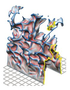
Figure 6.15: Instantaneous isotherm from the DNS of Bell et al. [261].
