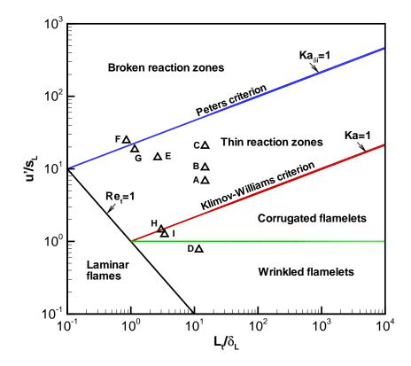
Figure 6.1: Turbulent premixed combustion regime diagram of Peters [113], showing the conditions of the cases that have been studied (empty triangles).
