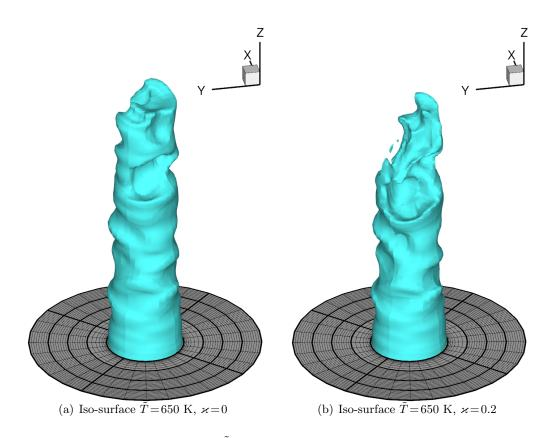
Figure 6.30: Instantaneous iso-surface  $\tilde{T} = 650$  K of the Bunsen-type flames at 56 ms. Left: CH<sub>4</sub>-air flame. Right: H<sub>2</sub>-CH<sub>4</sub>-air flame.
