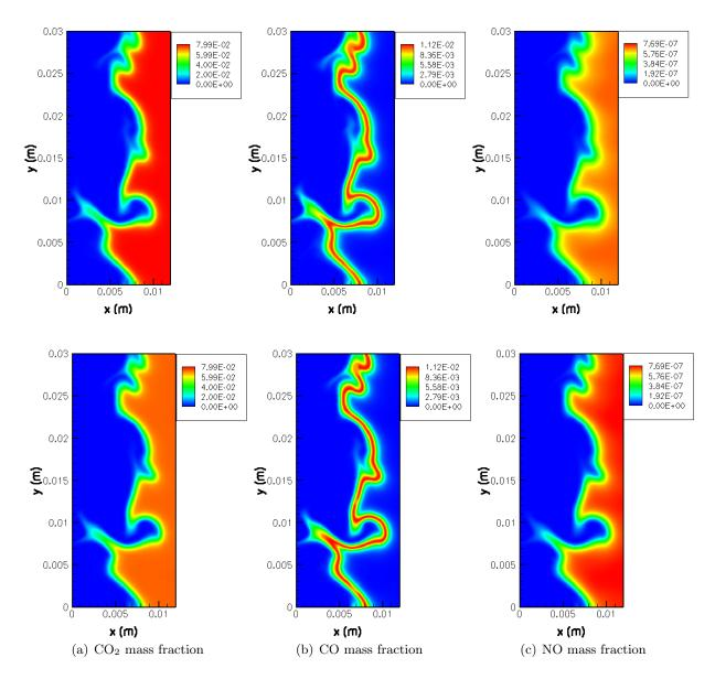
Figure 6.27: Predicted CO<sub>2</sub>, CO, and NO mass fraction contours of 2D freely-propagating flames at time t=3.0 ms. Top: CH<sub>4</sub>-air flame. Bottom: H<sub>2</sub>-CH<sub>4</sub>-air flame with 29% H<sub>2</sub> in the blended fuel.
