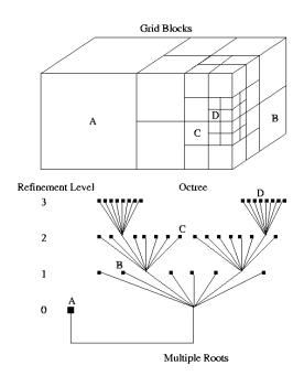
Figure 5.4: Multi-block hexahedral AMR mesh showing solution blocks at various levels of refinement and the corresponding octree data structure [246].
