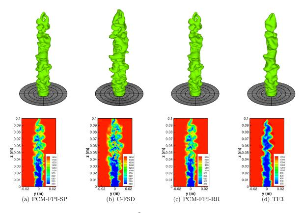
Figure 6.20: Instantaneous flame iso-surface  $\tilde{T} = 1076$  K at 4 ms after the initiation of the simulations. Bunsen burner configuration.
