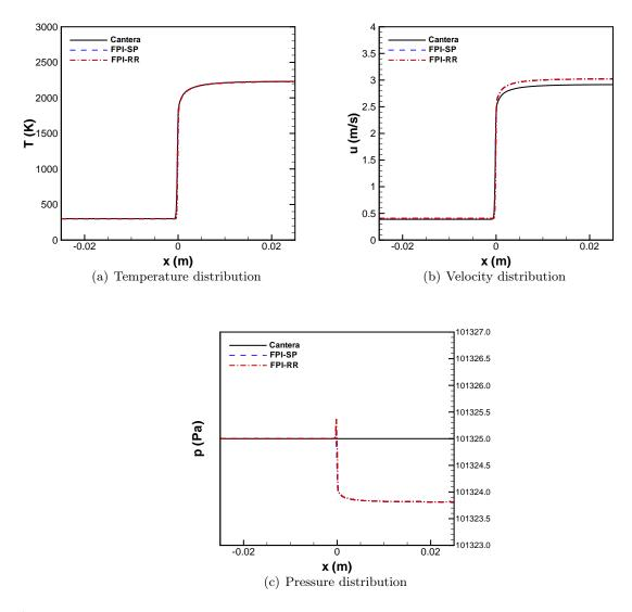
Figure 6.4: Temperature, velocity and pressure distributions of 1D steady-state stoichiometric methane-air flames.
