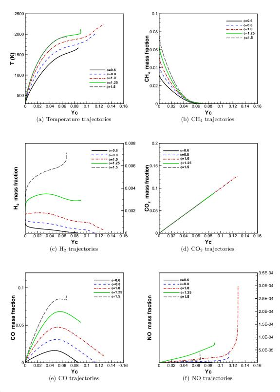
Figure 4.5: Temperature and representative species trajectories in the progress of reaction space for  $Y_c = Y_{CO_2} + Y_{NO}$ , corresponding to lean, stoichiometric, and rich conditions, and 20% H<sub>2</sub> in the blended H<sub>2</sub>-CH<sub>4</sub> fuel. 1D steady-state laminar premixed flames.
