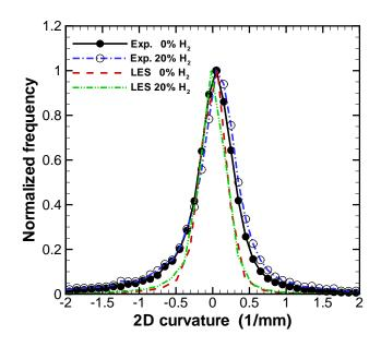
Figure 6.36: PDF of 2D curvature corresponding to a progress variable  $c_{\rm T} = 0.5$  for the Bunsen-type CH<sub>4</sub>-air and H<sub>2</sub>-CH<sub>4</sub>-air flames.
