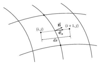
Figure 5.1: Weighted cell-face gradient approach for a two-dimensional grid.
