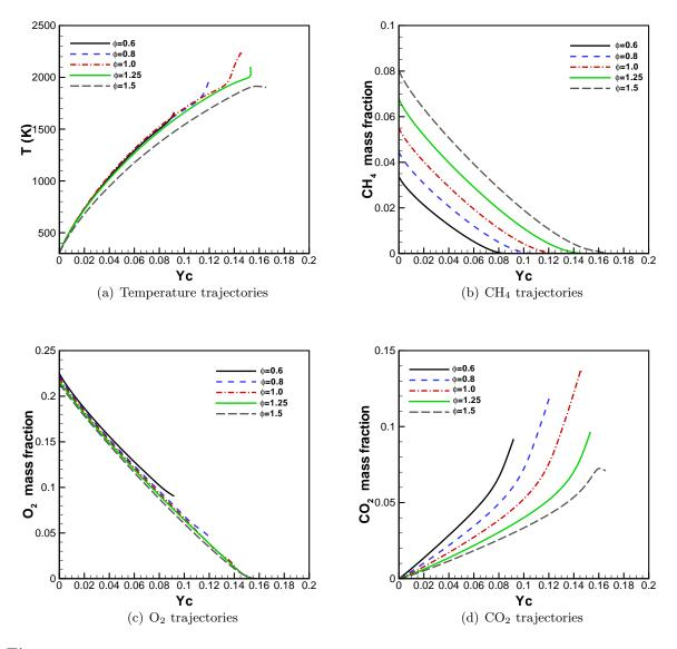
Figure 4.1: Temperature and representative species trajectories in the progress of reaction space for  $Y_c = Y_{CO_2} + Y_{CO}$ , corresponding to lean, stoichiometric, and rich conditions.
