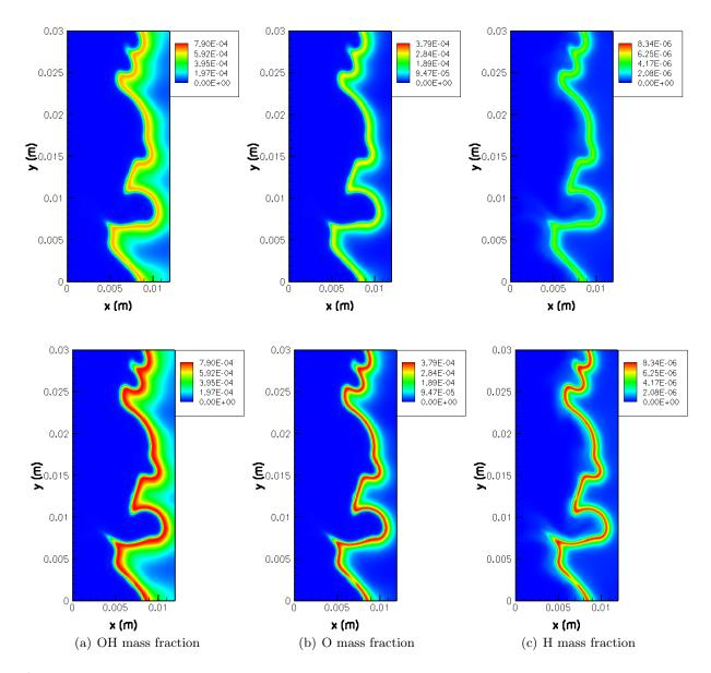
Figure 6.28: Predicted OH, O, and H mass fraction contours of 2D freely-propagating flames at time t=3.0 ms. Top: CH<sub>4</sub>-air flame. Bottom: H<sub>2</sub>-CH<sub>4</sub>-air flame with 29% H<sub>2</sub> in the blended fuel.
