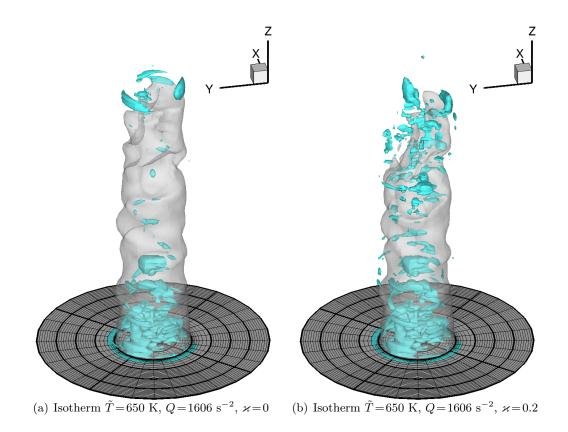
**Figure 6.31:** Instantaneous iso-surface  $\tilde{T} = 650$  K of the Bunsen-type flames (light grey) interacting with vortical structures (cyan) identified by  $Q = 0.5(u'/L_t)^2 = 1606$  s<sup>-2</sup> at 56 ms. Left: CH<sub>4</sub>-air flame. Right: H<sub>2</sub>-CH<sub>4</sub>-air flame.
