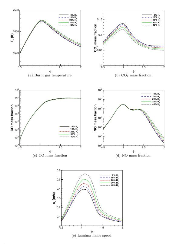
Figure 4.3: Influence of  $H_2$  addition on the burnt gas temperature, mass fractions of species  $CO_2$ , CO, and NO, and laminar flame speed. 1D steady-state laminar premixed flame solutions obtained using Cantera.
