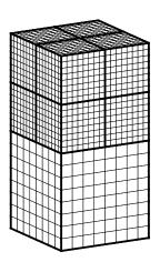
Figure 5.2: An example of two neighbouring  $8 \times 8 \times 8$  hexahedral solution blocks. One has undergone refinement [246].
