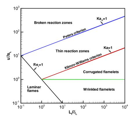
Figure 2.4: Diagram of turbulent premixed combustion regimes [113].
