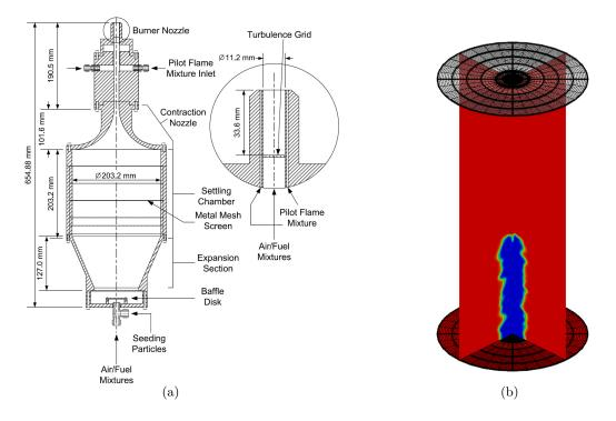
Figure 6.19: (a) Premixed Bunsen burner schematic [265]. (b) Computational domain for the premixed Bunsen flame.
