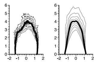
Figure 6.17: Flame brushes corresponding to the experiment and DNS [261] of the slot burner configuration. The thick lines correspond to the  $\langle c_{\rm T} \rangle = 0.5$  contour. The dimensions are in cm.
