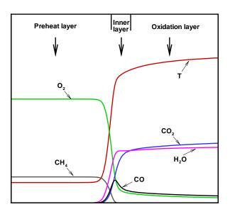
Figure 2.2: Structure of a 1D CH<sub>4</sub>-air flame.
