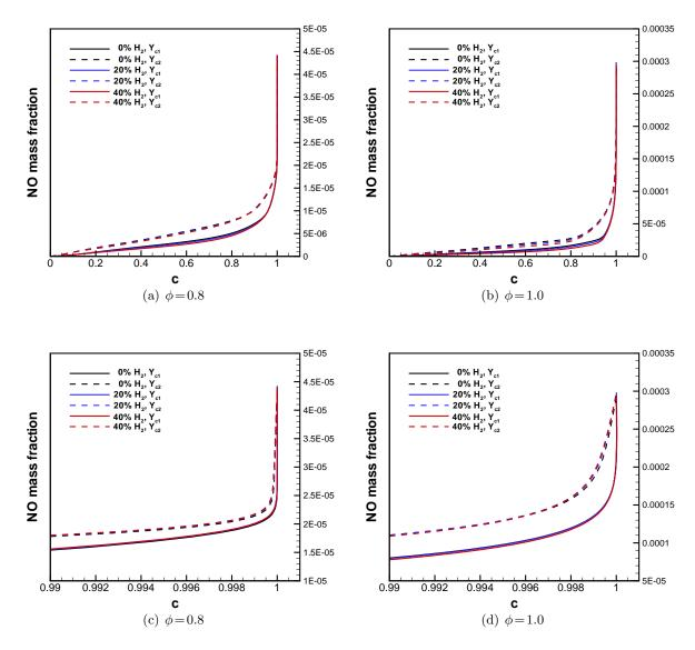
**Figure 4.4:** NO mass fraction evolution in the progress variable space for  $Y_{c1} = Y_{CO_2} + Y_{CO}$  and  $Y_{c2} = Y_{CO_2} + Y_{NO}$ , corresponding to lean and stoichiometric conditions ( $\phi = 0.8$  and  $\phi = 1.0$ ) with different levels of H<sub>2</sub> (0%, 20%, and 40% on a molar basis) in the blended H<sub>2</sub>-CH<sub>4</sub> fuel. 1D steady-state laminar premixed flames. Bottom: magnified views of the regions where NO is reaching its equilibrium value.
