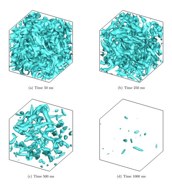
Figure 6.9: Q-criterion iso-surfaces corresponding to  $Q = 115 \text{ s}^{-2}$  at 50, 250, 500, and 1000 ms. Decay of homogeneous isotropic turbulence case.
