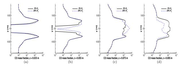
Figure 6.38: Radial profiles of the time-averaged CO mass fraction distribution of the Bunsen-type flames. Plane x=0.
