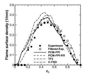
Figure 6.22: 2D Flame surface density extracted from the experimental data and LES simulations. Bunsen burner configuration.
