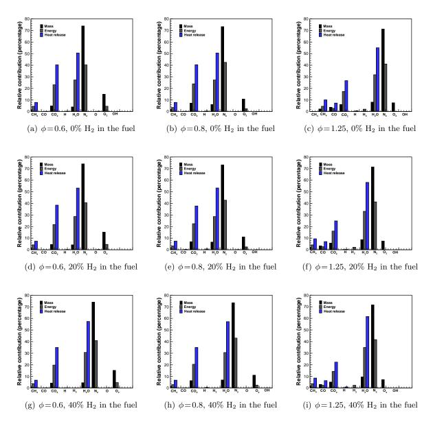
Figure 4.6: Relative mass, energy, and heat release contributions of the most representative species in H<sub>2</sub>-enriched methane-air premixed flamelets at equivalence ratios  $\phi = 0.6$ ,  $\phi = 0.8$ , and  $\phi = 1.25$ .
