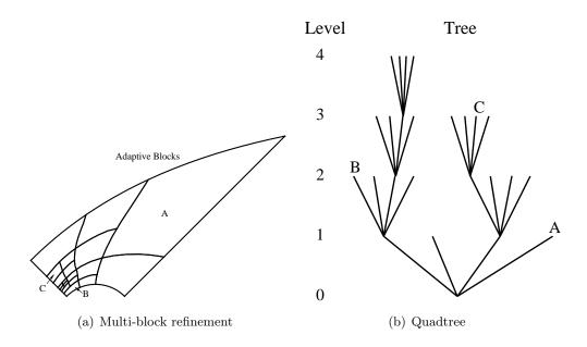
Figure 5.3: Multi-block quadrilateral AMR mesh showing solution blocks at various levels of refinement and the corresponding quadtree data structure [246].
