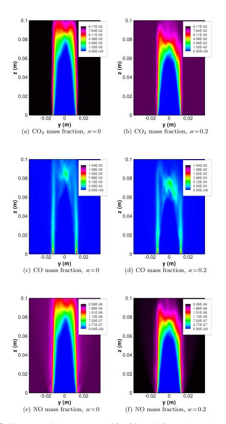
Figure 6.37: Planar cuts of the time-averaged CO<sub>2</sub>, CO, and NO mass fraction distributions of the Bunsen-type flames. Plane x=0. Left: CH<sub>4</sub>-air flame. Right: H<sub>2</sub>-CH<sub>4</sub>-air flame.
