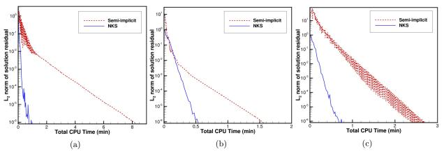
Figure 6: Comparison of convergence of the solution residuals for the NKS and semi-implicit solvers when applied to a Couette flow case with a Knudsen number of (a) 0.01, (b) 0.1, and (c) 1.
