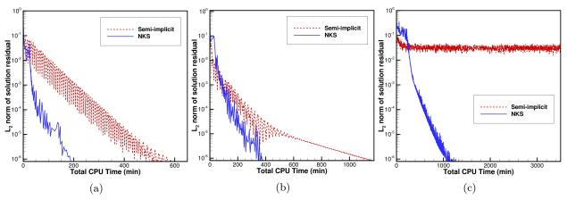
Figure 17: Comparison of solution convergence using the NKS and semi-implicit schemes for the circular cylinder case with a Knudsen number of (a) 0.01, (b) 0.1, and (c) 1 and a speed ratio of S=0.027.
