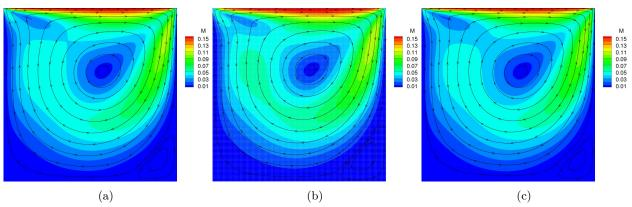
Figure 20: Mach number contours for lid-driven cavity flow at Kn = 0.001 found using the (a) regularized Gaussian closure, (b) 14-moment closure, and (c) NSF equations.
