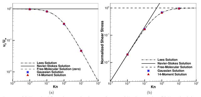
Figure 5: (a) Normalized flow velocity at the plate as a function of Knudsen number. (b) Normalized shear stress between the plates as a function of Knudsen number.
