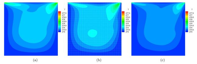
Figure 21: Temperature contours for lid-driven cavity flow at Kn = 0.001 found using the (a) regularized Gaussian closure, (b) 14-moment closure, and (c) NSF equations.
