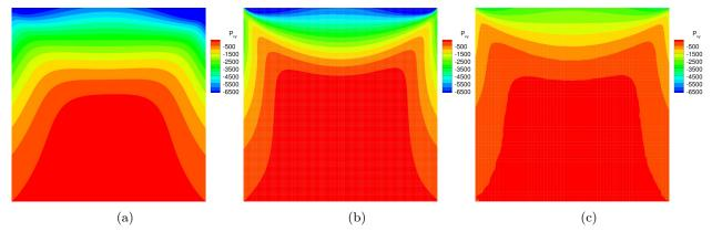
Figure 26: Shear stress contours for lid-driven cavity flow at Kn = 0.1 found using the (a) regularized Gaussian closure, (b) 14-moment closure, and (c) DSMC technique.<sup>59,60</sup>
