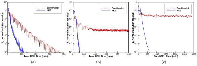
Figure 18: Comparison of solution convergence using the NKS and semi-implicit schemes for the circular cylinder case with a Knudsen number of (a) 0.01, (b) 0.1, and (c) 1 and a speed ratio of S=0.107.
