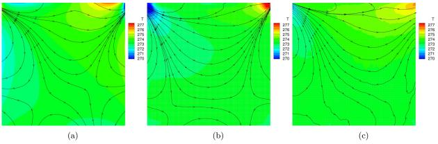
Figure 24: Temperature contours and heat-flux streamlines for lid-driven cavity flow at Kn = 0.05 found using the (a) regularized Gaussian closure, (b) 14-moment closure, and (c) DSMC technique.<sup>59,60</sup>
