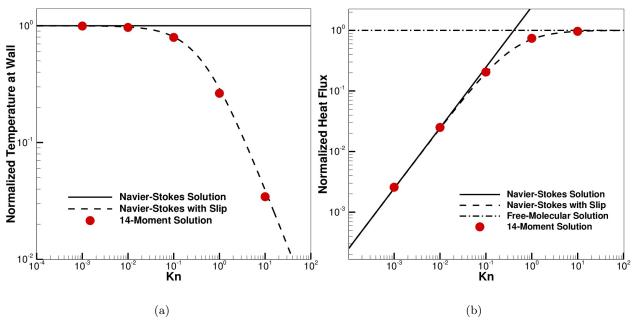
Figure 7: (a) Normalized temperature at the wall with respect to Knudsen number. (b) Heat flux between the plates, normalized with respect to the free-molecular value, as a function of Knudsen number.
