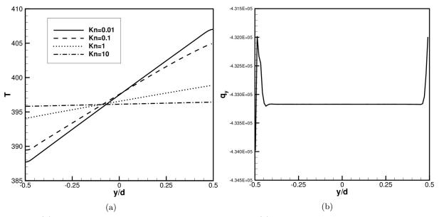
Figure 9: (a) Temperature distributions between heated plates. (b) Heat flux between heated plates at Kn=1.
