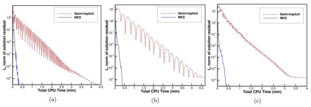
Figure 8: Comparison of convergence of the solution residuals for the NKS and semi-implicit solvers when applied to a heated flat plates case with a Knudsen number of (a) 0.01, (b) 0.1, and (c) 1.
