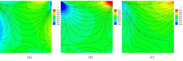
Figure 27: Temperature contours and heat-flux streamlines for lid-driven cavity flow at Kn = 0.1 found using the (a) regularized Gaussian closure, (b) 14-moment closure, and (c) DSMC technique.<sup>59,60</sup>
