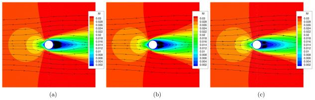
Figure 11: Mach number contours and velocity streamlines for subsonic flow past a circular cylinder at Kn = 0.002 found by solving the (a) Gaussian, (b) regularized Gaussian, and (c) 14-moment closures.
