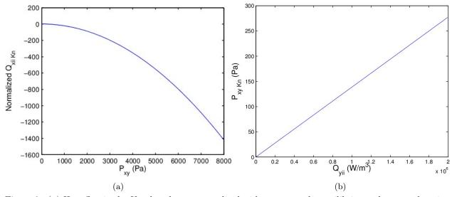
Figure 2: (a) Heat flux in the Knudsen layer, normalized with respect to the equilibrium value, as a function of the shear pressure in the interior fluid. (b) Shear pressure in the Knudsen layer as a function of heat flux parallel to the boundary. The remaining interior fluid properties are set to typical values for argon gas.
