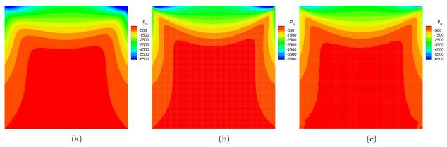
Figure 23: Shear stress contours for lid-driven cavity flow at Kn = 0.05 found using the (a) regularized Gaussian closure, (b) 14-moment closure, and (c) DSMC technique.<sup>59,60</sup>
