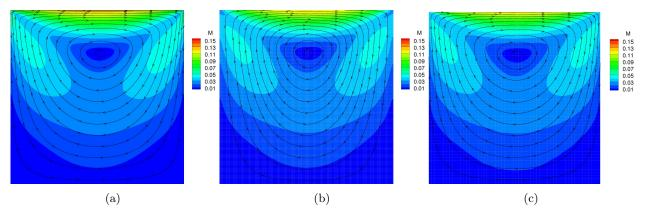
Figure 22: Mach number contours for lid-driven cavity flow at Kn = 0.05 found using the (a) regularized Gaussian closure, (b) 14-moment closure, and (c) DSMC technique.<sup>59,60</sup>
