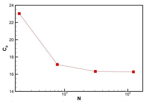
Figure 10: Mesh refinement study for subsonic flow around a circular cylinder at Kn=0.1 and S=0.027. N is the total number of computational cells.
