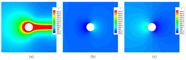
Figure 14: Temperature contours for subsonic flow past a circular cylinder at Kn = 1 found by solving the (a) Gaussian, (b) regularized Gaussian, and (c) 14-moment closures.
