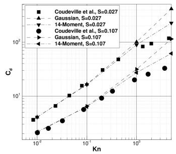
Figure 16: Comparison of predicted drag coefficients found using the 14-moment and Gaussian closures and experimental values for air found by Coudeville et al..
