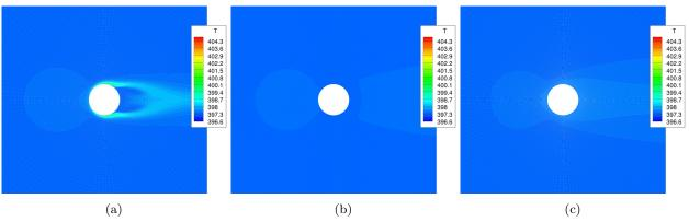
Figure 12: Temperature contours for subsonic flow past a circular cylinder at Kn = 0.002 found by solving the (a) Gaussian, (b) regularized Gaussian, and (c) 14-moment closures.
