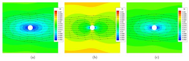
Figure 13: Mach number contours and velocity streamlines for subsonic flow past a circular cylinder at Kn = 1 found by solving the (a) Gaussian, (b) regularized Gaussian, and (c) 14-moment closures.
