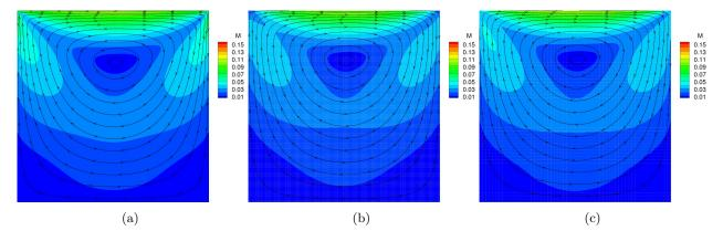
Figure 25: Mach number contours for lid-driven cavity flow at Kn = 0.1 found using the (a) regularized Gaussian closure, (b) 14-moment closure, and (c) DSMC technique.<sup>59,60</sup>
