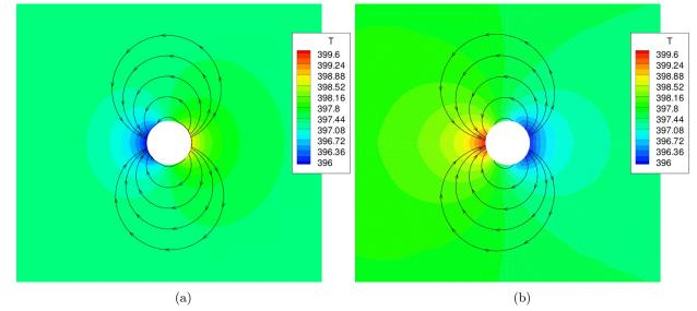
Figure 15: Temperature contours and heat-flux streamlines for subsonic flow past a circular cylinder at Kn = 1 found by solving the (a) regularized Gaussian and (b) 14-moment closures. Note that the temperature contours have been rescaled to show more detail.
