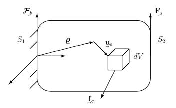
We consider a contrained elastic body with volume V. Impressed on V is a body force distribution (per unit volume)
