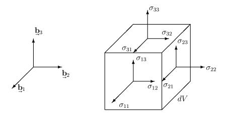
The notation  $\sigma_{ij}(\boldsymbol{\rho})$ , i, j = 1, 2, 3 denotes the stress tensor.  $\sigma_{11}, \sigma_{22}$ , and  $\sigma_{33}$  are normal stresses and  $\tau_{ij} = \sigma_{ij}, i \neq j$ , are shear stresses. It can be shown that  $\sigma_{ij} = \sigma_{ji}$ .
